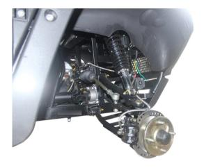
Smart brakes - Front and rear hydraulic disc brakes feature an intelligent Energy Recovery System to provide additional braking power and increase driving range. During braking and steep descents the energy recovery system converts the vehicles kinetic energy to electricity that is used to recharge the intelligent battery system.
